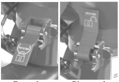
Engaged Disengaged Fig. 14 Left-right Lock Indication
